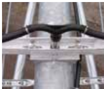
The Senninger Double Gooseneck attaches to the 3/4" x 4" galvanized nipple through a pre-drilled hole in the aluminum channel and into an existing outlet.
